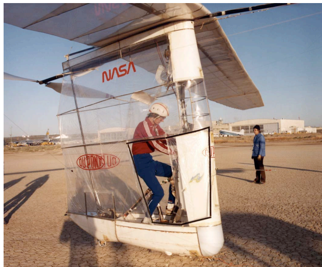
Bryan Allen, about to pedal the Gossamer Albatross, with its 96 foot wingspan. It weighed only 66 pounds. Allen was both the pilot and the engine. (NASA photo by Jim Moran)
